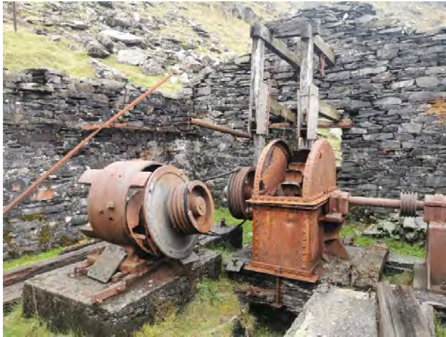
Pelton wheel and generator
