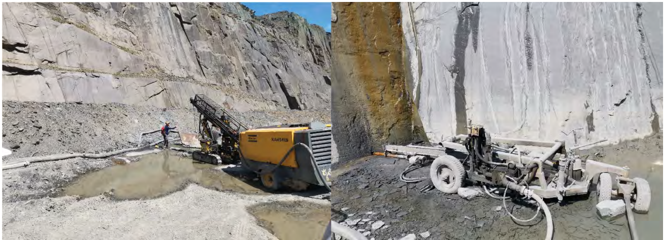
Carls further explanations of the working in the bottom of the quarry and the horizontal drill in situ ready to start drilling again on the return to work.
