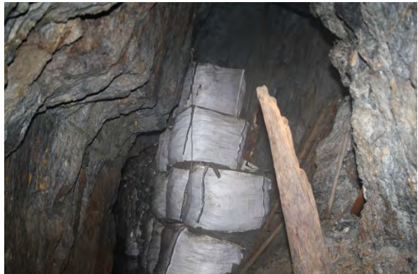
Building the pack wall to get rid of the debris
